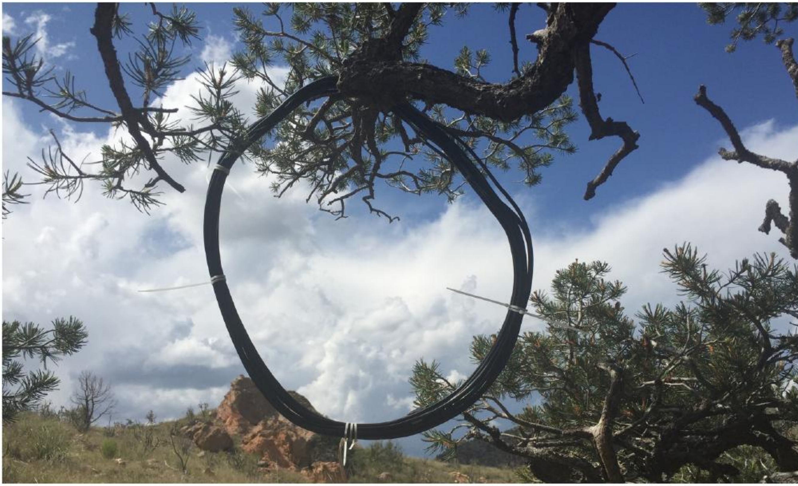
VLF Receiver made from eight-core signal cable and secured with cable ties by composer and media artist Thomas Rex Beverly, Ohio, USA
