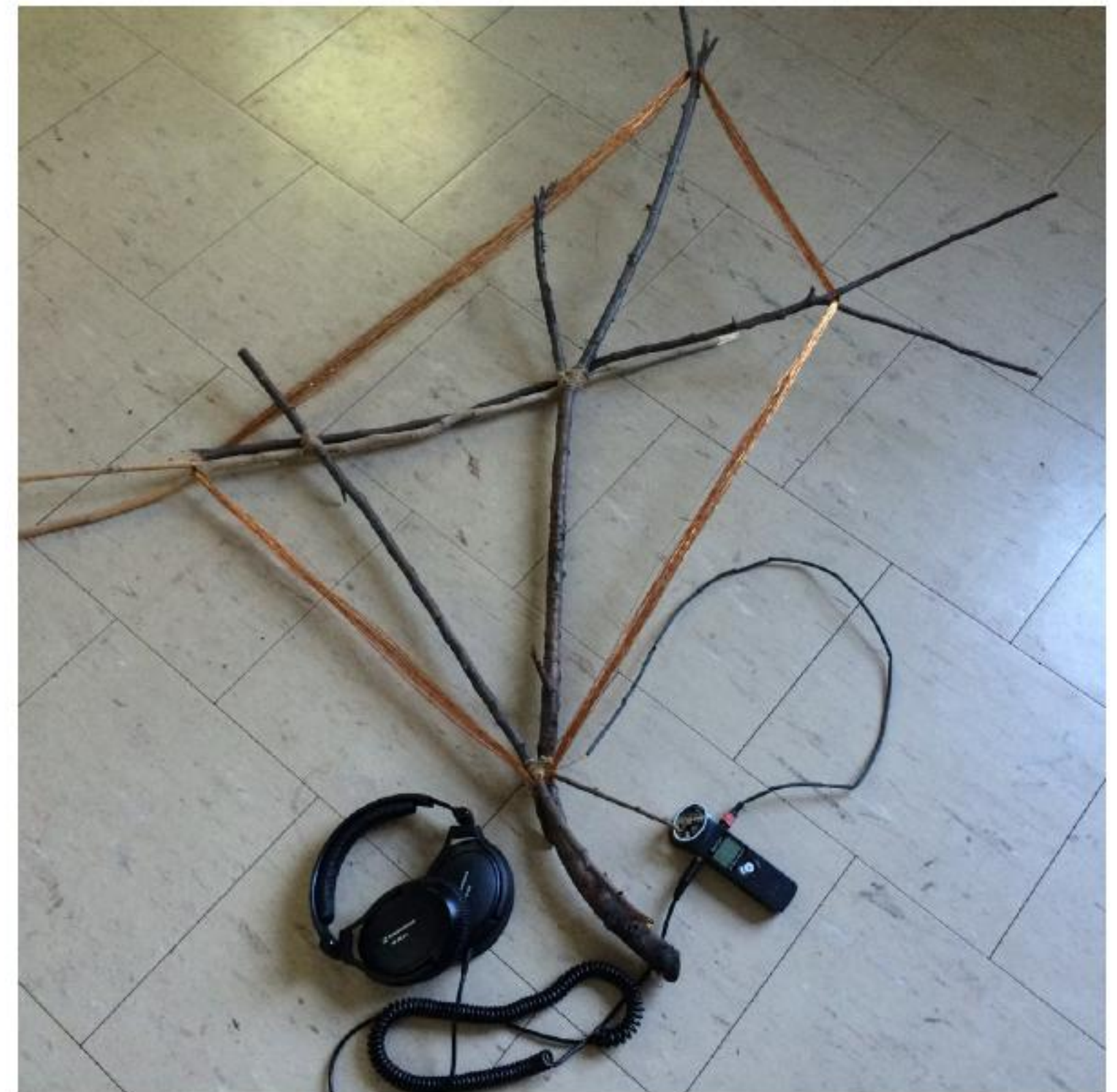
VLF receiver made from magnet wire and tree branches by sound artist Claude Wittman, Toronto, Canada
