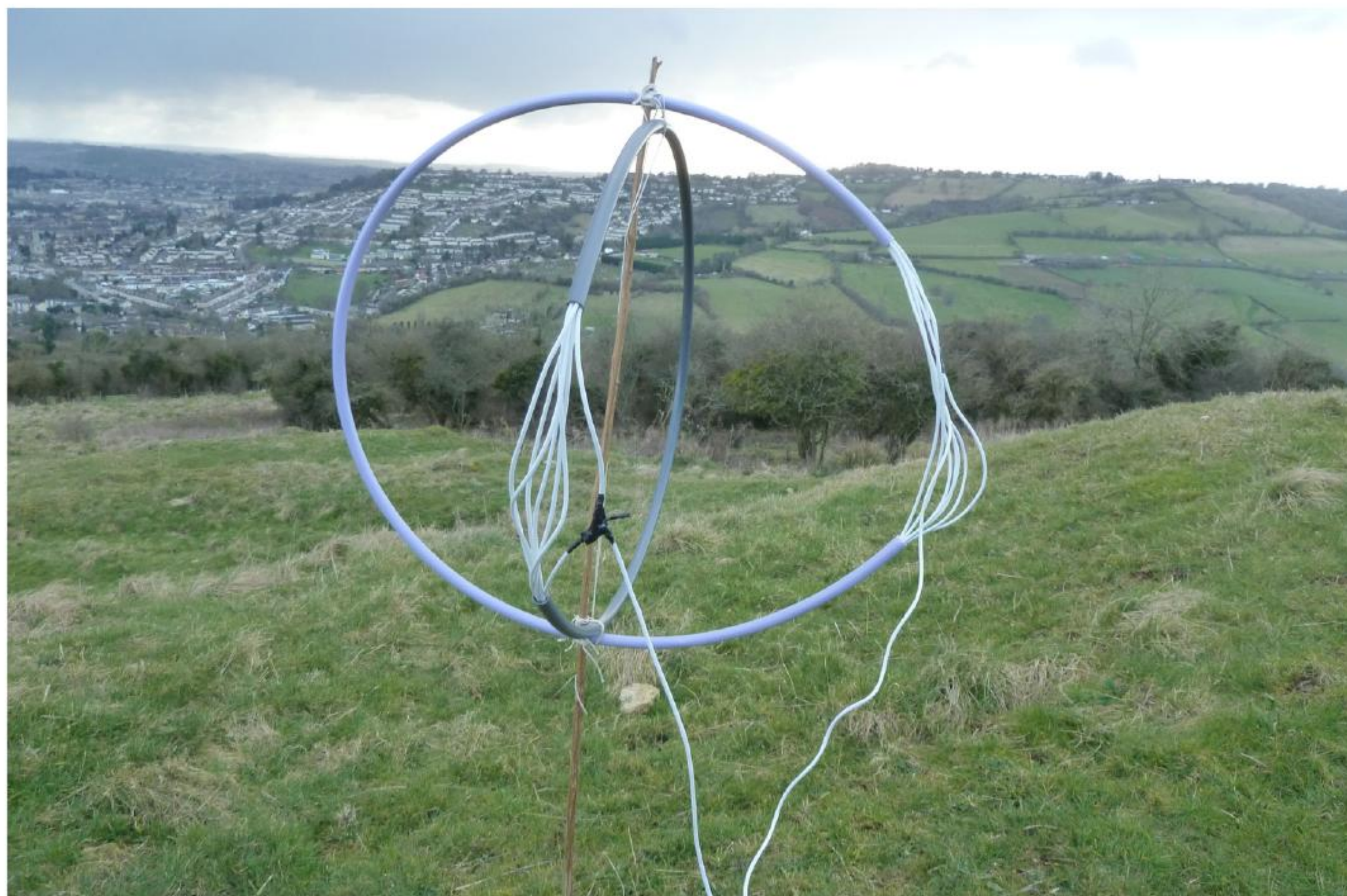
Two VLF receivers made from four-core signal cable and hula-hoops, with makeshift handle. made by Dan Tapper in Bath, UK.
