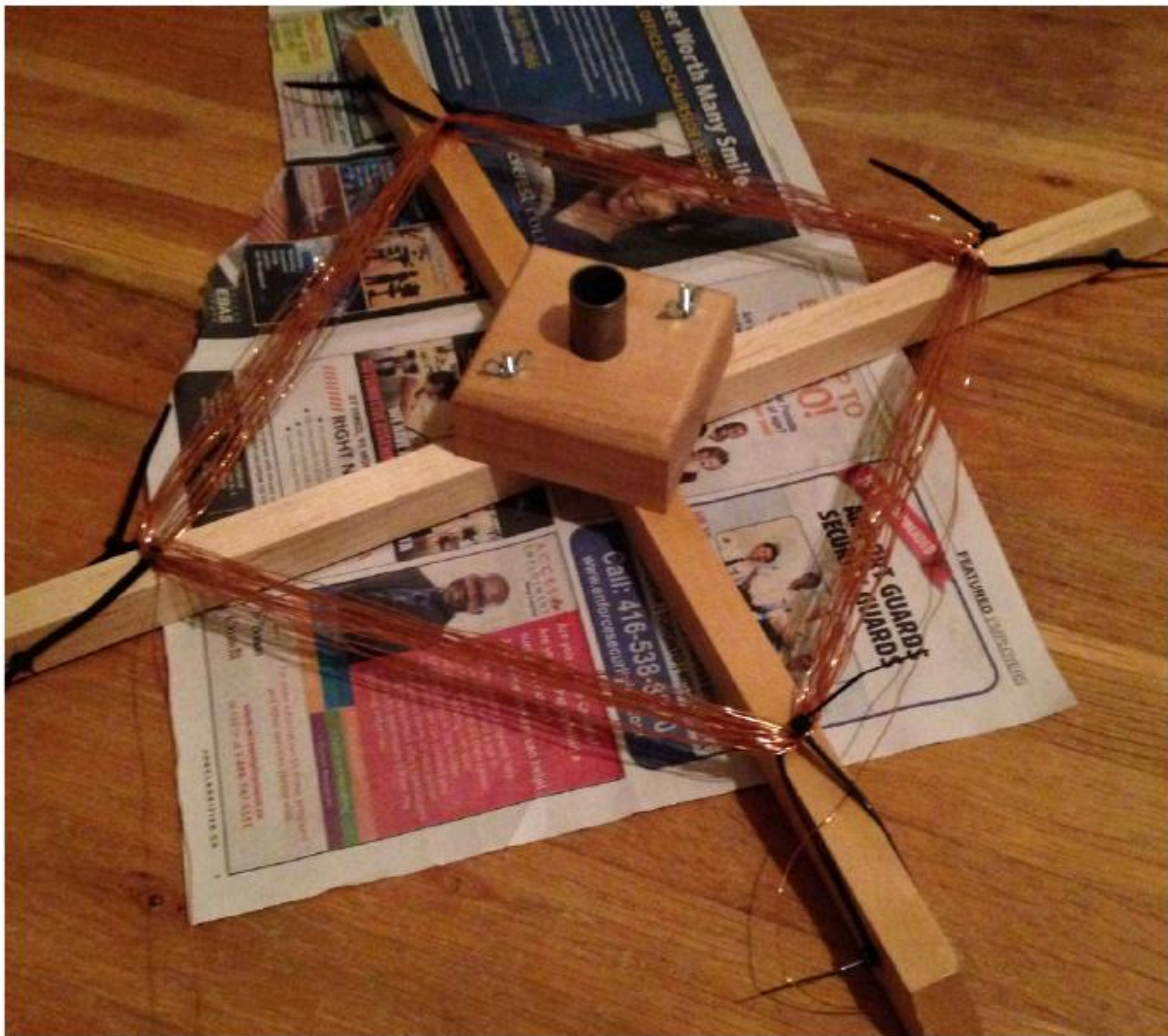
VLF receiver made from magnet wire and found wood. Made by Dan Tapper in Toronto, Canada
